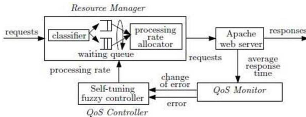
**Figure 11: System Architecture of Apache Server STFC**
