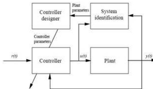
**Figure 6: Indirect Adaptive Control**
