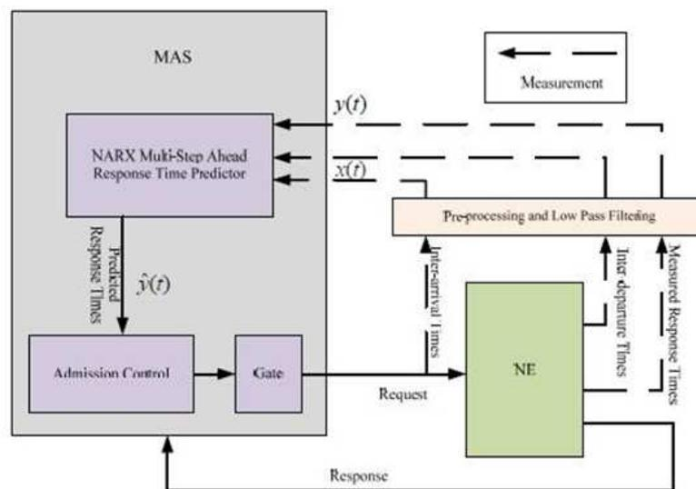
Figure 15: Mutli-Step Ahead Response Time Predictor
