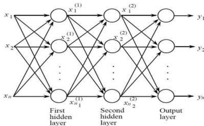
**Figure 2: A 3-Layer Multi Perceptron Model**
