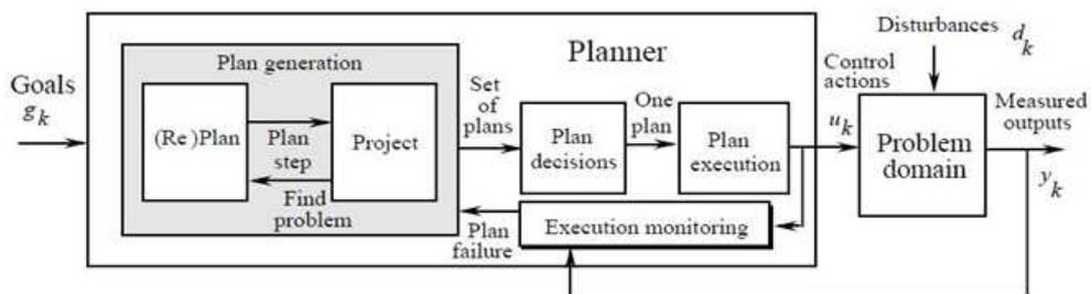
Figure 5: Closed Loop Planning Control System
