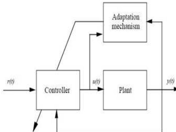
**Figure 7: Direct Adaptive Control**
