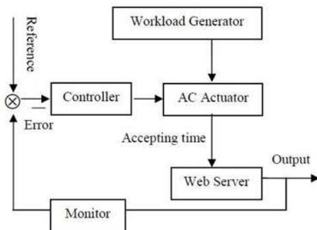
Figure 9: Architecture of ATR Feedback System
